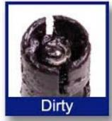
Fuel injector deposits at the injector tip can impact fuel flow, upsetting the air/fuel mixture. The symptoms of these deposits can be:
