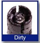
Fuel injector deposits at the injector tip can impact fuel flow, upsetting the air/fuel mixture. The symptoms of these deposits can be:
